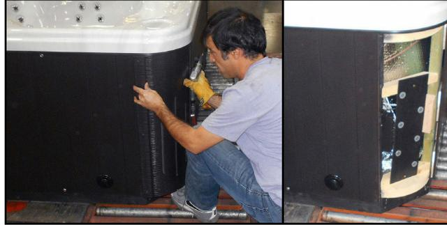
Unscrew and remove the two corner panels on each side of the spa's front door.
