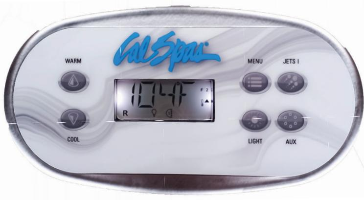
Some panels have separate WARM (Up) and COOL (Down) buttons, while others have a single Temperature button. In the navigation diagrams Temperature buttons are indicated by a single button icon.
