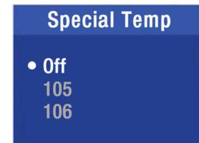
'Special Temp' will heat the spa one time to the selected temperature. The spa will then maintain the previous 'Set Temperature'.
